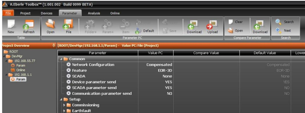
Figure 56: Starting parameter upload to the device
