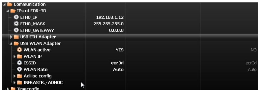
Figure 61: USB Wi-Fi adapter configuration
