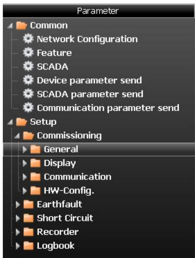
Figure 34: Tree structure of the Parameter menu (example)
